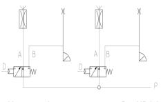
D = Air connectionA = Outlet flow divider P = HP inlet B = Outlet gun
